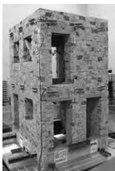
Figure 9. Masonry model, reinforced using injections, on the shaking table (Mazzon et al., 2009).
