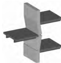
Figure 10. Floors at different height in adjacent U.S. The seismic action can push on the common wall.
