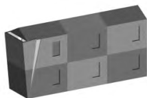
Figure 8. The U.S. in head position is not buttressed by the other buildings.
