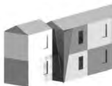
Figure 7. The not aligned facade causes a wall not to be buttressed by the other buildings.
