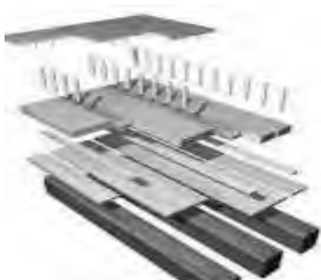
Figure 12. In-plane and Out-of-plane stiffening of an existing wooden floor: wooden planks at the extrados connected by wooden dowels.
