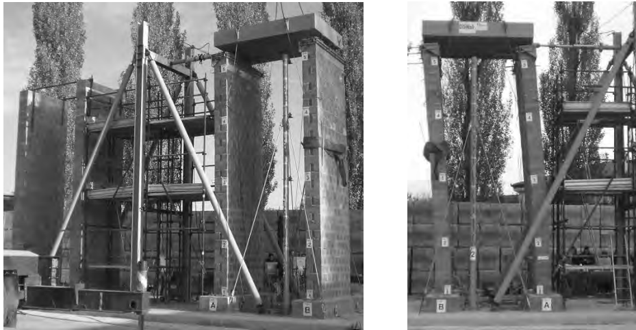
Figure 3. Cyclic out-of-plane tests on reinforced masonry walls. Left: view of the test set-up; right: final deflection for the walls with 0.13% vertical reinforcement (Mosele et al. 2008; Mosele 2009).
