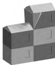
Figure 9. Adjacent U.S. of different height. It may be possible the collapse of the higher one.
