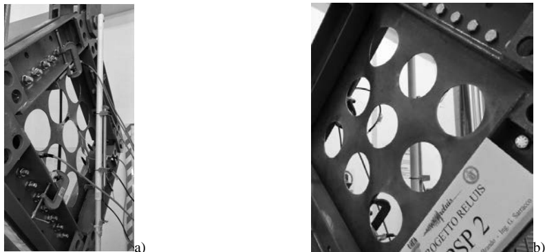
Figure 12. The first buckling phenomena revealed for (a) the specimen PSP1 at a displacement of \pm 5.00\text{ mm} (shear strain of \pm 1.1\% ) and (b) specimen PSP2 at a displacement of \pm 2.00\text{ mm} (shear strain of \pm 0.4\% ).
