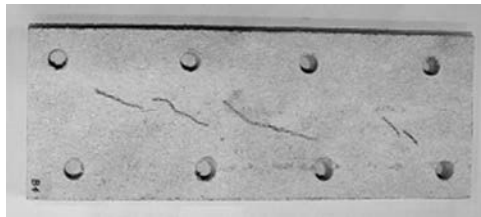
Figure 12. Example of collapse mode observed in a sheathing specimen.
