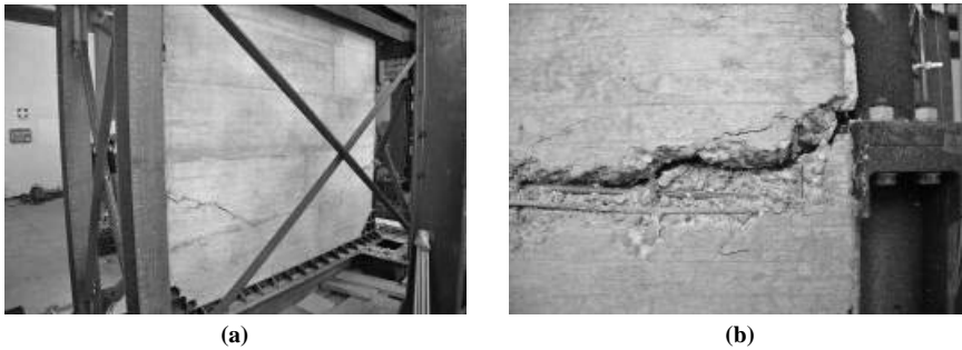
Figure 20. Specimen 2 at the end of the test: (a) global view; (b) failure of the steel reinforcements in tension crossing the main crack.
