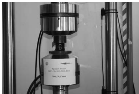
Figure 10. Compression tests on prototype recycled rubber isolators.
