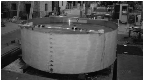
Figure 5. Mock-up of the above-ground tank.
