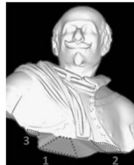
Figure 9. Bust of Marcantonio Eugeni by Francesco Mochi. Finding on the model from laser scan of the rest areas on the base.
