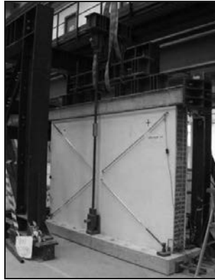
Figure 21. Full scale solid brick walls.
